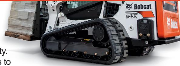
You don't have to sacrifice ride comfort for added traction. Bobcat tracks have been tested and proven to not only withstand the most challenging environments, but to also deliver a softer ride by distributing the machine's weight over a larger surface area. Our tracks offer the traction needed to bring out the loader's full capabilities. Wider and thicker roller path area is key to the tracks' improved performance and vibration-mitigating technology – even on worn rollers.
